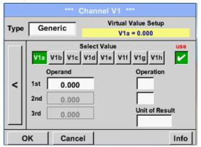
By accessing the text field 1st Operand The list with all channels (HW and virtual channels) and const. Value appears.
