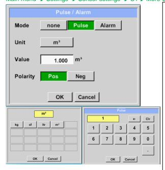
To set up the pulse first the unit and the measurement value have to be defined.
