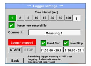
By pushing the *timed Stop* button and then the date/time description field below, the date and the stop time can be set for a data logger recording.
