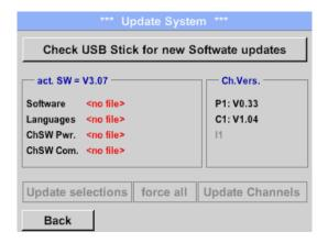
If after pushing the *Check USB Stick for new Software updates* button the following messages in the window appears, then DL 200 is not connected properly with the USB stick or no files are available.
