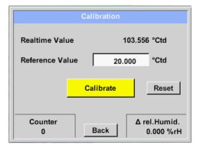
Here, a one-point calibration can be performed.
