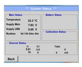
The function System Status offers an overview, fitting voltages and currents on the individual and the entire channel, as well as the power supply of the power supply unit.
