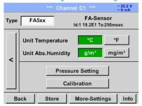
Unit selection for temperature and humidity by pressing the button °C, °F, g/m³ or mg/m³.
