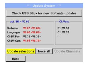
If the DL 200 is correctly connected to USB, and new version available it will displayed.
