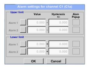
In the alarm settings, an *Alarm 1* and *Alarm 2* incl. *Hysteresis* can be entered for each channel.
