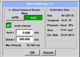
In *More-Settings*, you can define whether the 4 - 20 mA analogue output of the sensor based on the flow rate or velocity.
