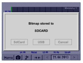
After pressing the Screenshot button a menu (see left) appears where the storage target, USB Stick or internal SD-card, could be selected.
