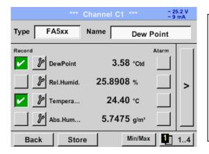
The connection with the FA 5xx sensor is done after confirmation by pressing "OK".
