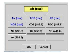
All gases marked in blue and with (real) have been a real gas calibration curve stored in the sensor.
