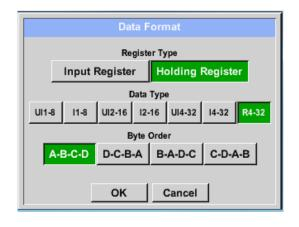
With the buttons *Input Register* and *Holding Register* the corresponding Modbus-register type will be selected.
