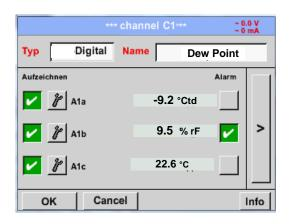
The DL 200 detects, if the connected sensor is a flow or dew point sensor and set the Digital subtype automatically correct.
