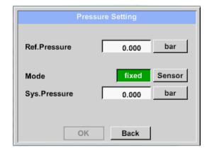
By using an ext. pressure sensor, which is detected automatically e.g. here at input B1, the button *Sensor* has to be activated.
