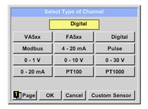
Now the *Type Digital* is selected for the VA/FA 400 series and confirmed by pressing the *OK* button.
