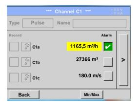
Like in Main Real time values, individual channels can be selected here, to detect which and how much the value has exceeded or below the alarm range.
