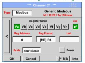
The measurement values are kept in the registers of the sensor and can be addressed via Modbus and read by the DL 200
