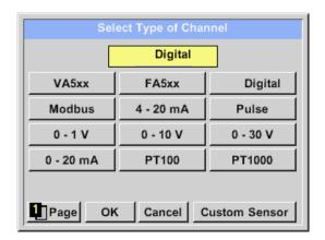
Now the *Type CS-Digital* is selected for the VA/FA 400 series and confirmed by pressing the *OK* button.
