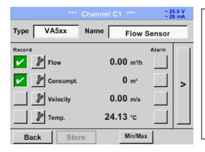
The connection with the VA 5xx sensor is done after confirmation by pressing "OK".
