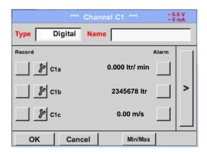
The DL 200 detects, if the connected sensor is a flow or dew point sensor of **CS Instruments** and set the CS-Digital subtype automatically correct.
