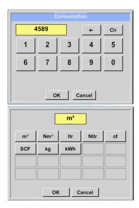
The sensor allows taking over a starting counter value. Inserting the value by entering the "Count. Val." text field.
