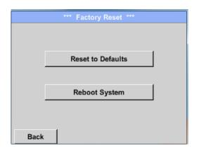
If necessary or required, by pressing the *Reboot System*-button the DL 200 could be rebooted.
