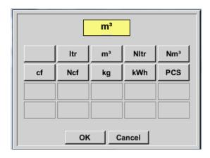
By *Unit Pulse* you can choose between a flow volume or a power consumption unit.
