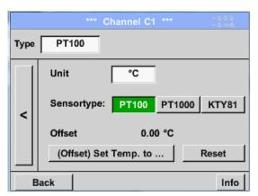
Here the sensor type PT100 and the Unit in °C are chosen, alternatively the sensor types PT1000 and KTY81, as well as the Unit °F can be selected.
