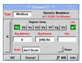
Via Modbus, it is possible to read out up to 8 Register-Values (from Input or Holding Register) of the sensor.
